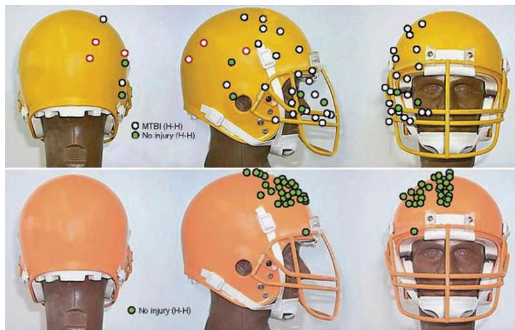
FIGURE 2. Photographs showing location of initial helmet contacts for the struck players (top, both concussive and nonconcussive impacts) and striking players (bottom, none of whom were concussed). All of the strikes in the plot are shown on the right side of the helmet to visualize the impacts, although the game impacts occurred on both sides of the helmet. MTBI (H-H) indicates a concussed player involved in a helmet-to-helmet impact (modified from, Pellman EJ, Viano DC, Tucker AM, Casson IR, Waekerle JF: Concussion in professional football: Reconstruction of game impacts and injuries. Neurosurgery 53:799-814, 2003 [39] by removing the helmet-to-ground impacts).
