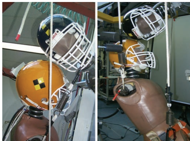
FIGURE 1. Photographs showing reconstruction of game impacts in laboratory tests with instrumented dummies (left, Test 39, and right, Test 162). The torso and pelvis of the striking player were suspended from below, and the struck player was simulated with the head and neck attached to a 7.1 kg drop weight. Adjustments were made in the setup to duplicate the helmet kinematics in the game impact. The tests involved VSR-4 helmets by Riddell.
